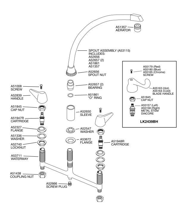
Warning: Blade handles must only be used with A55157 and A55158 Metal Stem Diacore Cartridges.
